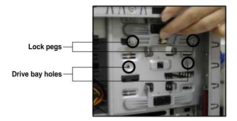
While holding up the bar lock, carefully insert a 5.25-inch drive into the bay, until the back of the drive aligns to the rear edge of the drive cage.
